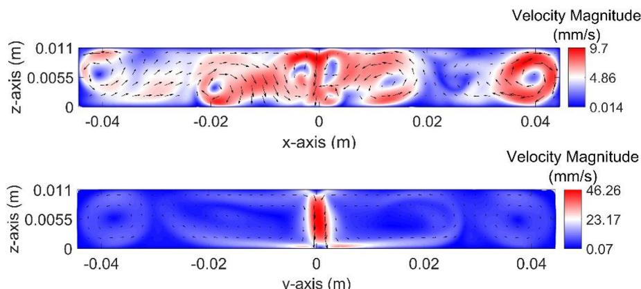
Figure – Rayleigh-Bénard convection and Electro-vortex flow in a PbBi electrode with current supplied at densities equivalent to a LMB discharging at  $0.25 \text{ A/cm}^2$  (top) and  $1 \text{ A/cm}^2$  (bottom)
